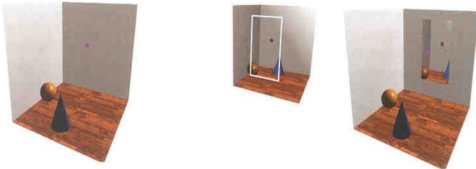
Figure 17.4 Masking reflections using projective texture.
